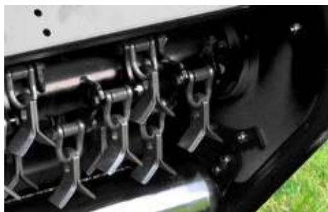
Y-shaped mounting of knives on shackles
