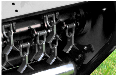
Y-shaped mounting of knives on shackles
