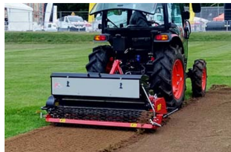
SMC 130 on soil preparator RD 130
