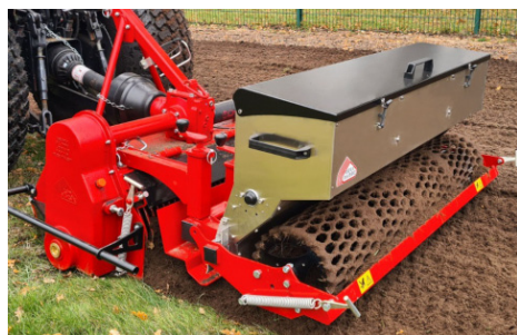
SG 130 on soil preparator RD 130
