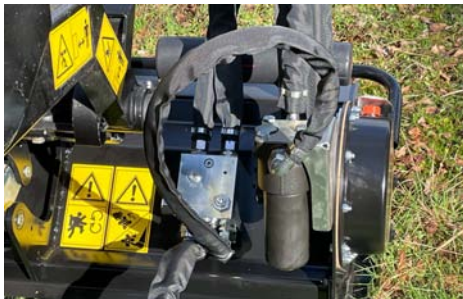
Safety hydraulic block with Cartridge filtration
