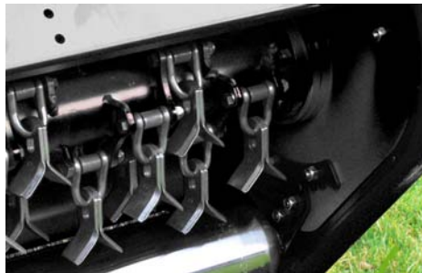
Y-shaped mounting of knives on shackles
