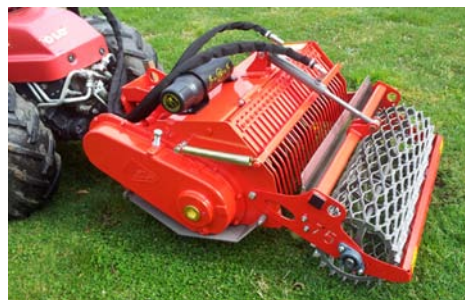
Option : Working depth setting by hydraulic jack
