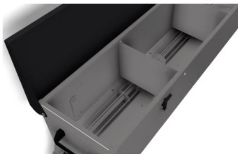
Mixer for decompacting seeds in the seedbox
