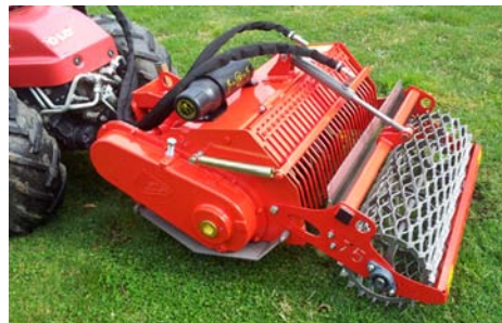
Option : Working depth setting by hydraulic jack
