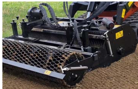
Option : Roller side adjustment device by cylinder
