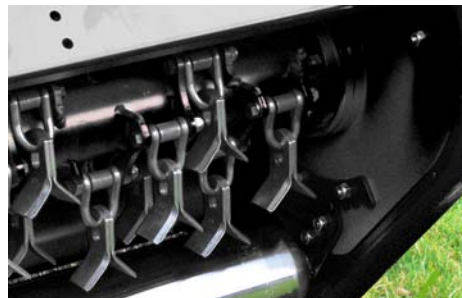
Y-shaped mounting of knives on shackles
