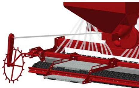
Access platform for the tank
