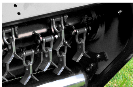
Y-shaped mounting of knives on shackles
