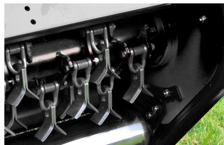
Y-shaped mounting of knives on shackles
