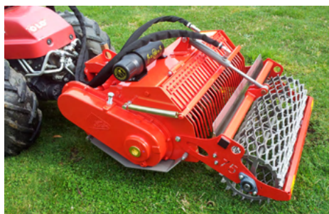
Option : Working depth setting by hydraulic jack
