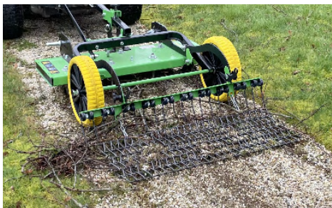
Rake, harrow and grid for clod crumbling
