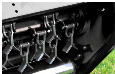
Y-shaped mounting of knives on shackles
