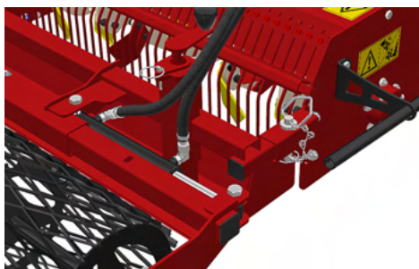
Option : Hydraulic movement of the mesh metal roller frame
