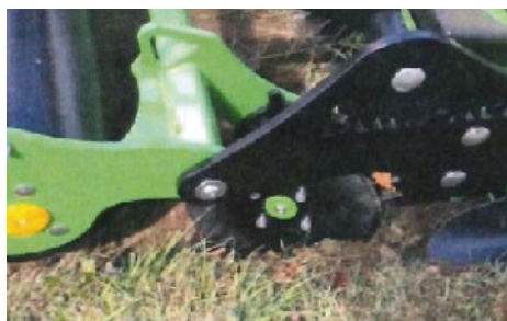
Option : edge trimming with sharpened disc
