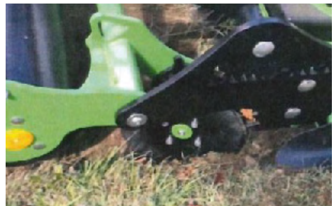
Option : edge trimming with sharpened disc
