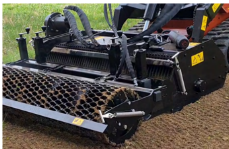
Option : Roller side adjustment device by cylinder
