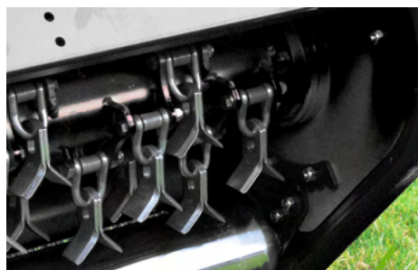
Y-shaped mounting of knives on shackles
