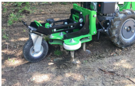
Cup-type cutting table patented
