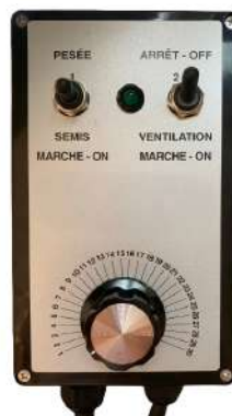
Seed flow adjustment via the graduated dial
