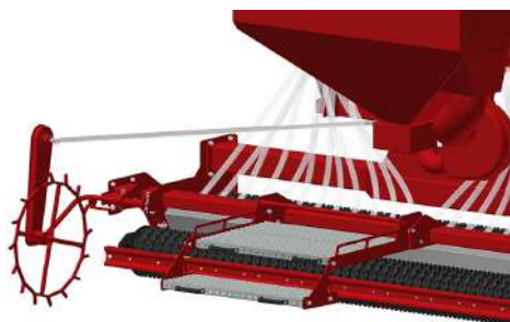
Access platform for the tank
