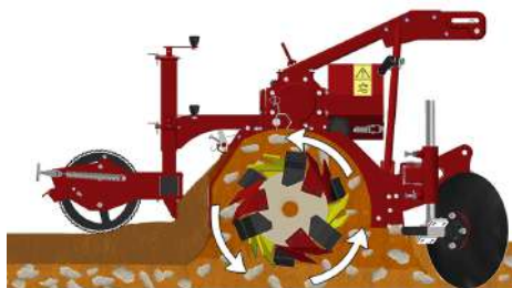
Soil preparation principle
