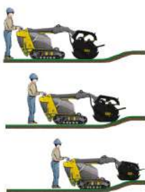
Floating field following system
