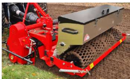
Option : Stainless Steel Gravity Grass Seeder SG on Stony 90 and Stony 115 (See SG P.56)
