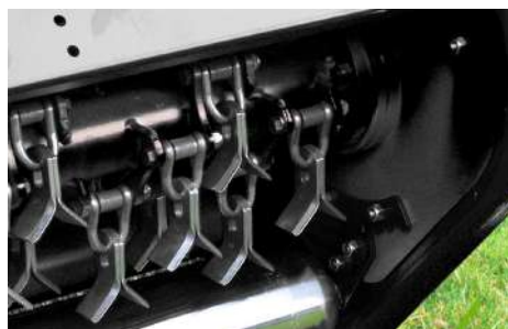
Y-shaped mounting of knives on shackles
