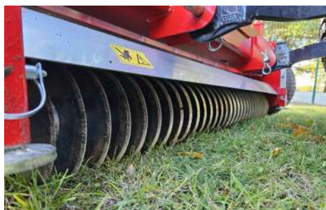
Sharp discs for stress action on weeds
