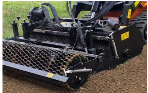
Option : Roller side adjustment device by cylinder
