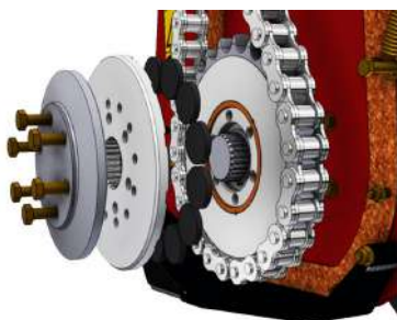
Oil bath torque limiter at the end of the rotor
