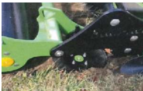
Option : edge trimming with sharpened disc
