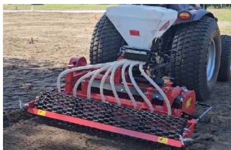
Option : Ventilated spline-slit seeder SCV (See P.56)
