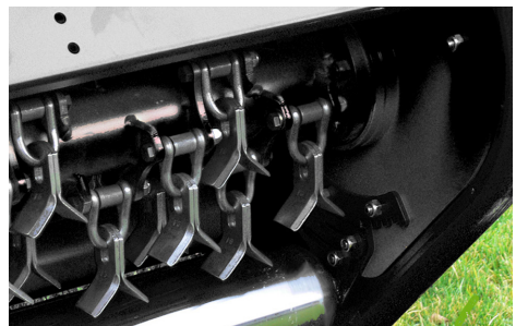
Y-shaped mounting of knives on shackles
