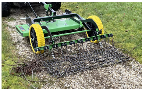
Rake, harrow and grid for clod crumbling
