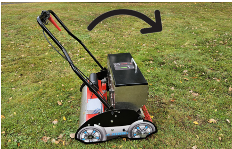
Handlebar in seeding position, tiltable to overseeding position
