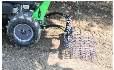
Finishing raking and harrowing
