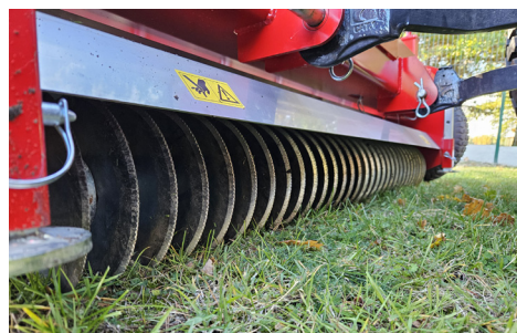
Sharp discs for stress action on weeds
