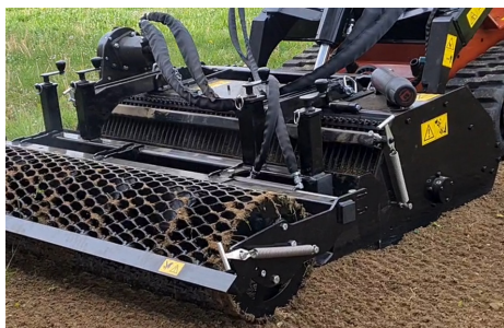
Option : Roller side adjustment device by cylinder
