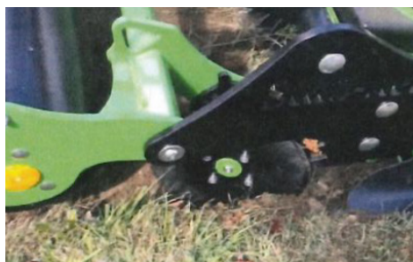
Option : edge trimming with sharpened disc
