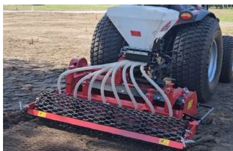
Option : Ventilated spline-slit seeder SCV (See P.56)
