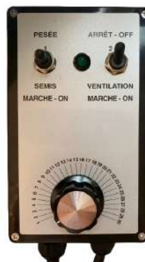
Seed flow adjustment via the graduated dial
