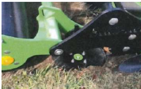
Option : edge trimming with sharpened disc
