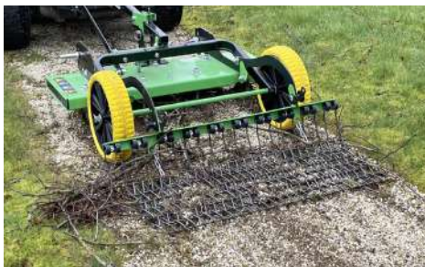
Rake, harrow and grid for clod crumbling
