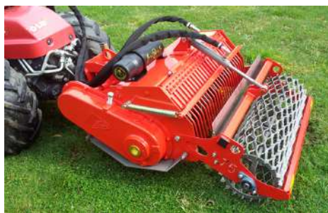
Option : Working depth setting by hydraulic jack
