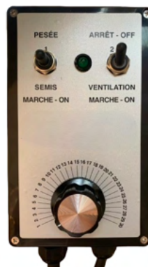
Seed flow adjustment via the graduated dial
