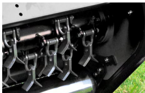
Y-shaped mounting of knives on shackles
