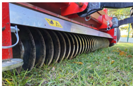
Sharp discs for stress action on weeds
