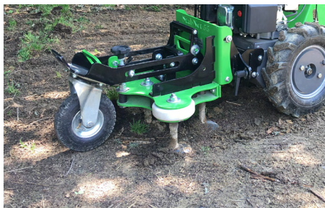
Cup-type cutting table patented
