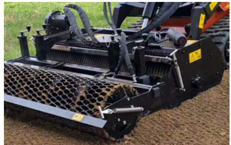
Option : Roller side adjustment device by cylinder
